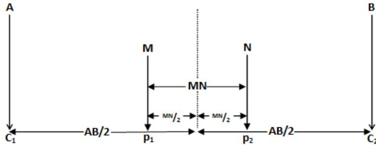
Figure 4: Schlumberger electrode configuration.
